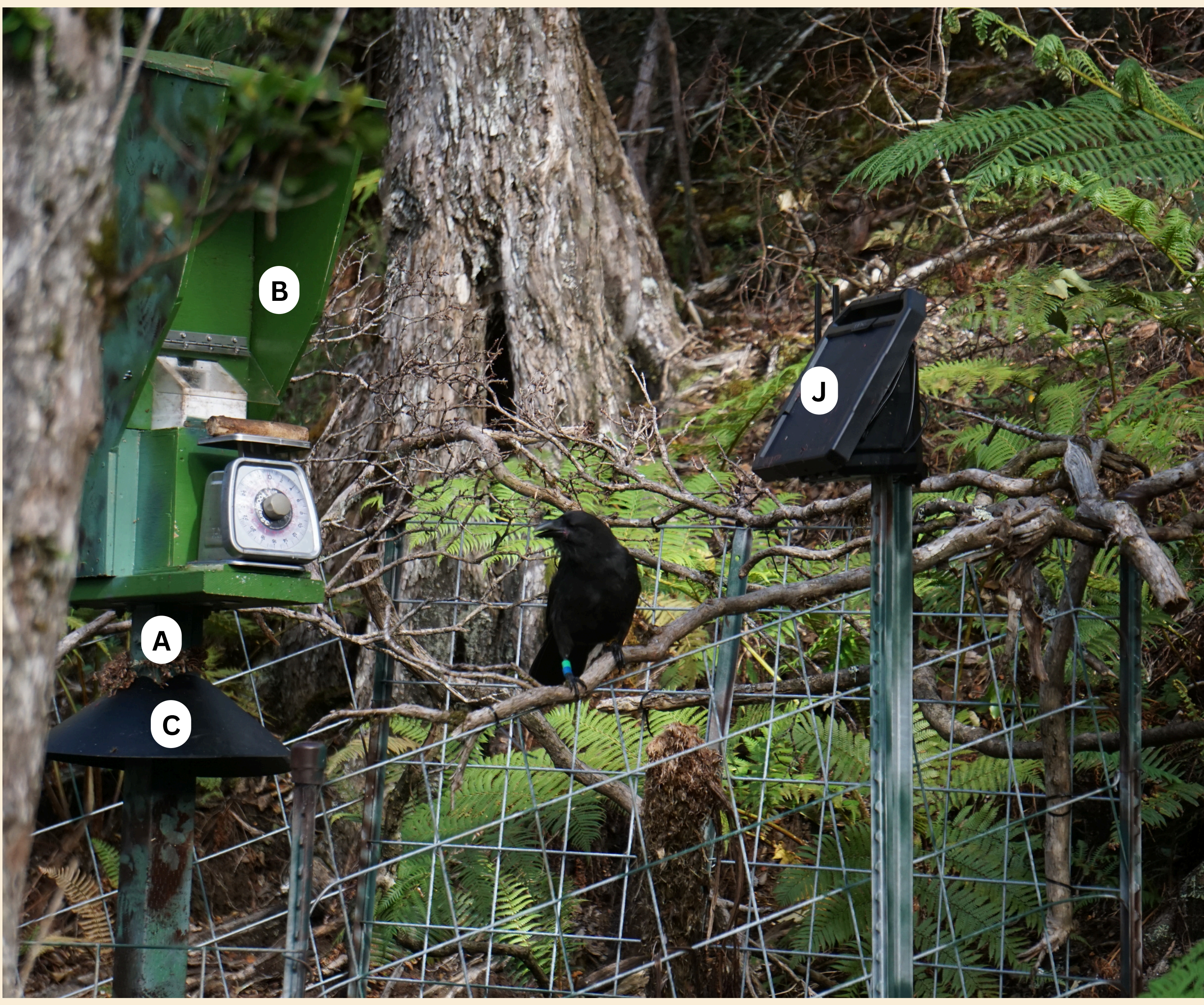
Figure 2: Alalā perched next to feeder at field site. A - stand, B - hale, C - rat baffle, J - cellular enabled game camera mounted with solar panel
