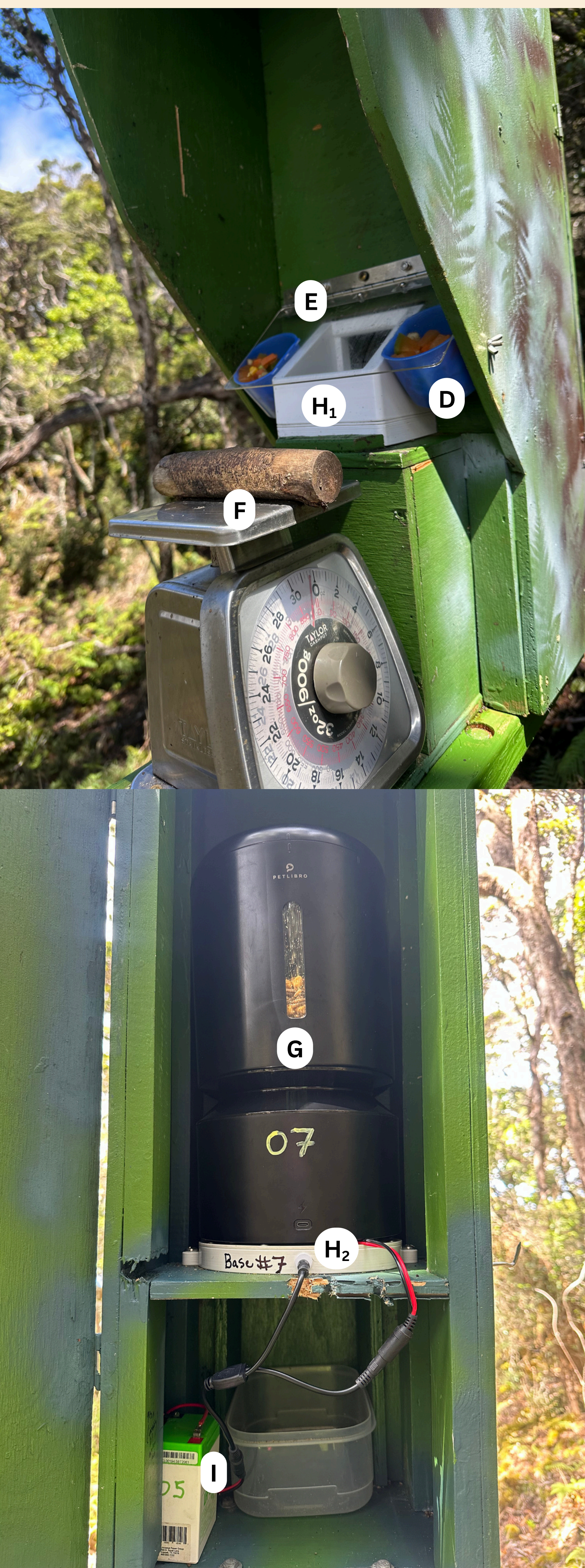
Figure 1: Feeder Hale exterior view (top) interior view (bottom). D - detachable blue cups, E - lid, F - scale with perch, G - repurposed automatic cat feeder, H 1 - hopper base front view, H 2 - hopper base interior view, I - 6V lithium battery
