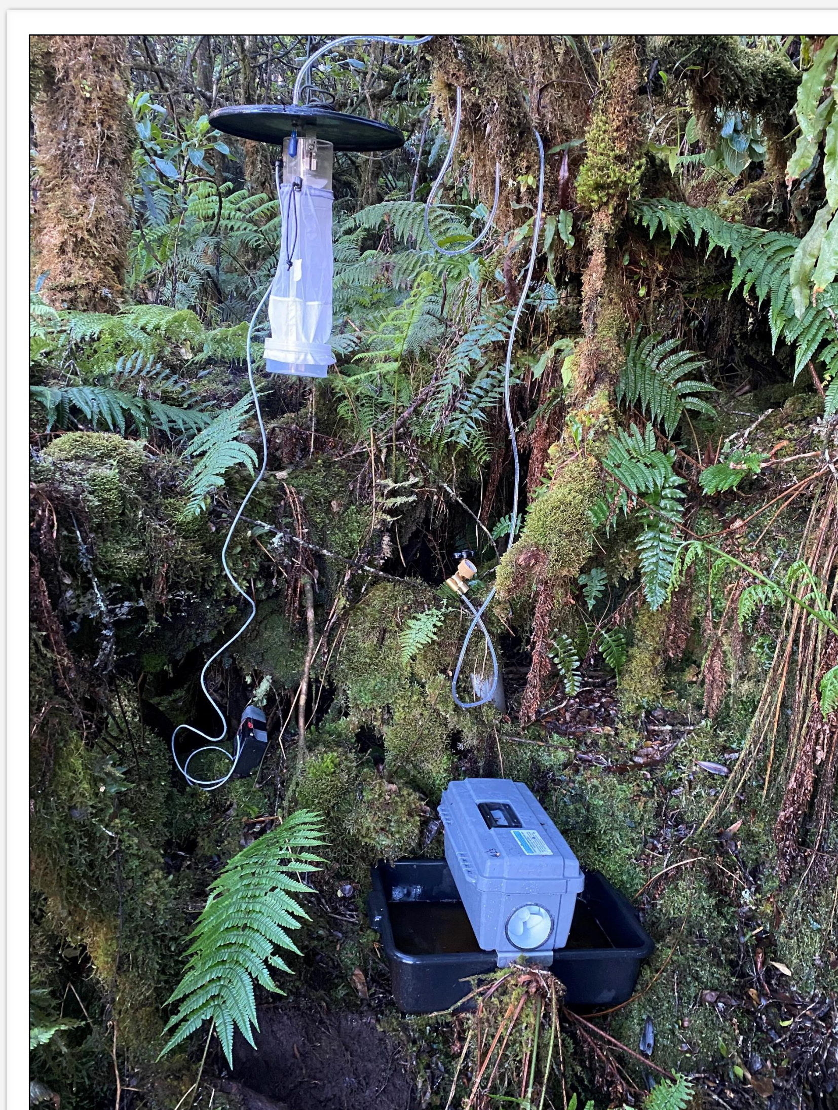
Figure 2. Above: Modified Centers for Disease Control and Prevention (CDC) light trap with CO 2 to target female mosquitoes looking for a blood meal. Below: Reiter-Cummings modified gravid trap with fetid water to target female mosquitoes looking to lay eggs.
