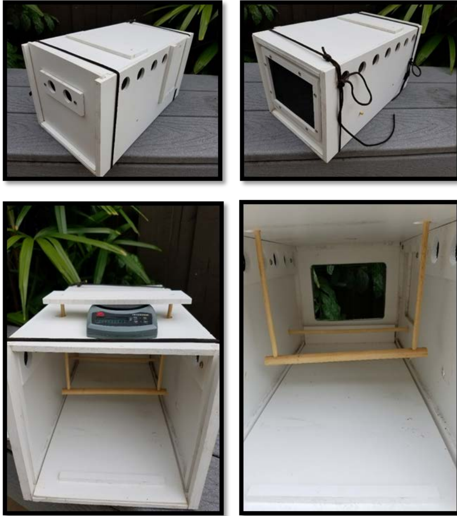
Figure 12. Single compartment holding cages used at the capture site camp with remote weighing system and removable perches and floor.
