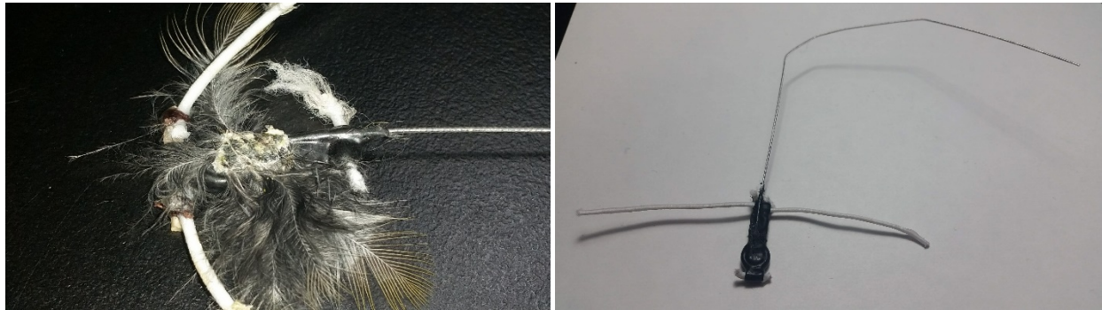
Figure 17. Photos of transmitters after they were removed from kiwikiu at Maui Bird Conservation Center. These photos show the most extreme examples of dead skin and feathers stuck to the ventral surface of the transmitter (left) and bent antenna (21-kg test wire) (right).
