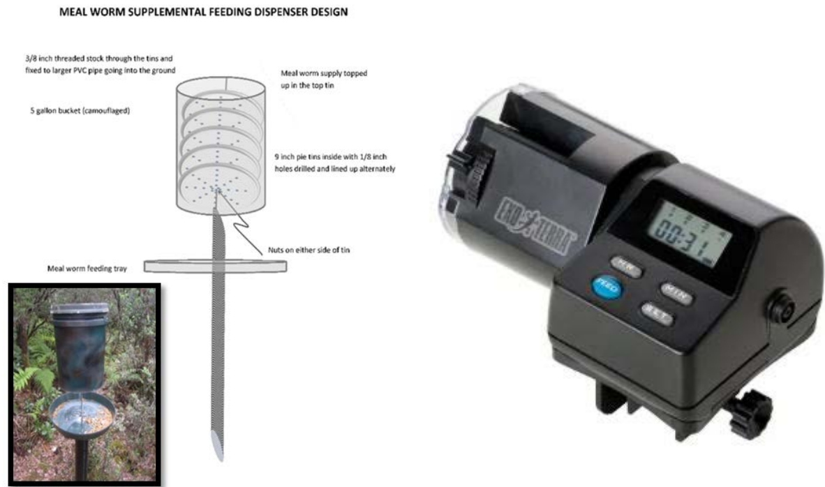
Figure 8. Supplemental feeder design (left) and Exo Terra® Turtle Feeder/Automatic Feeder Unit used to dispense dry pelleted food that was placed inside the bucket of the supplemental feeder.
