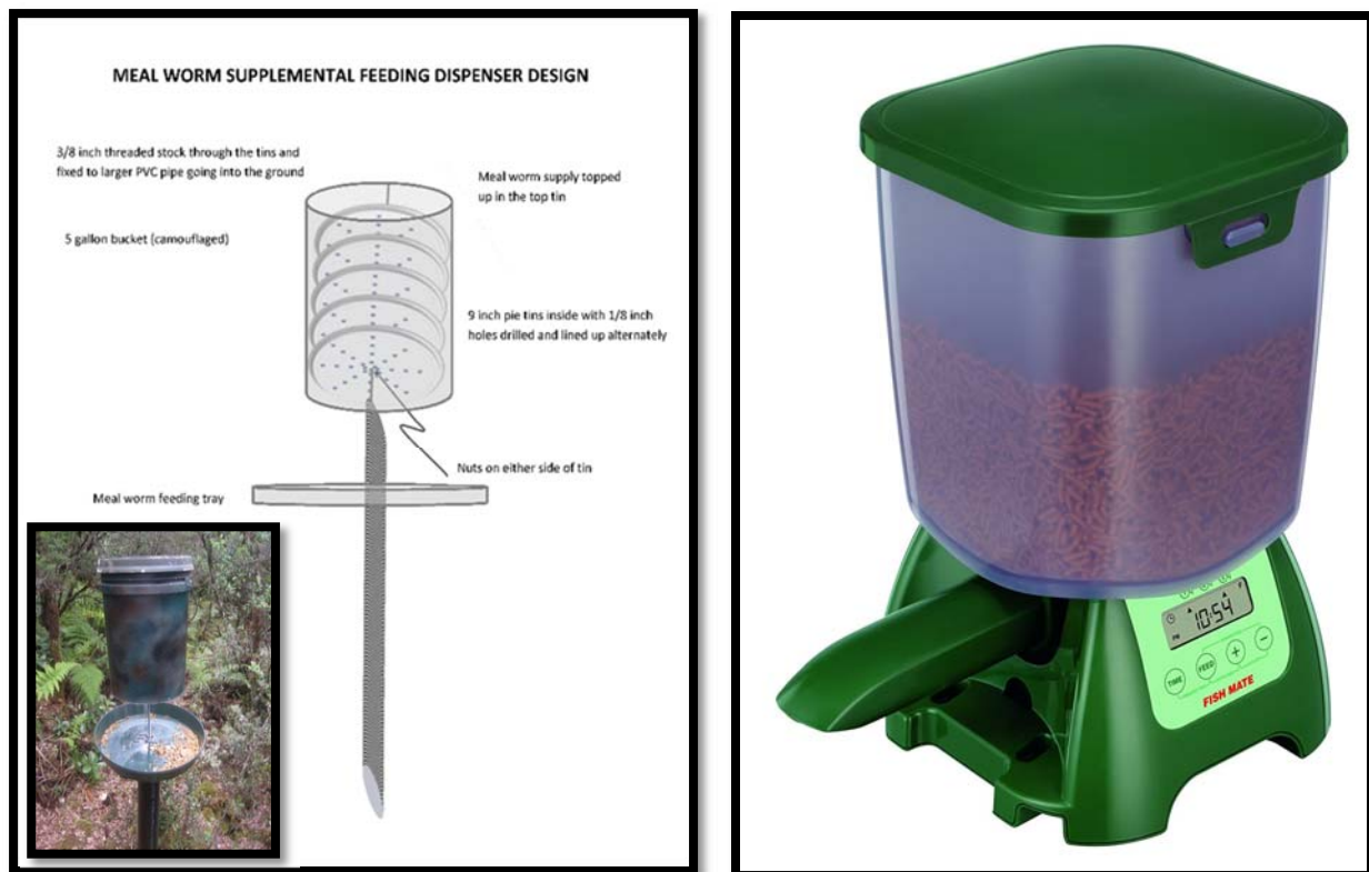
Figure 15. Prototype supplemental feeding dispenser designs to be placed inside each aviary cell and outside of the release aviary. The exact feeder used will be slightly different modification designed as a hybrid of the two pictured.
